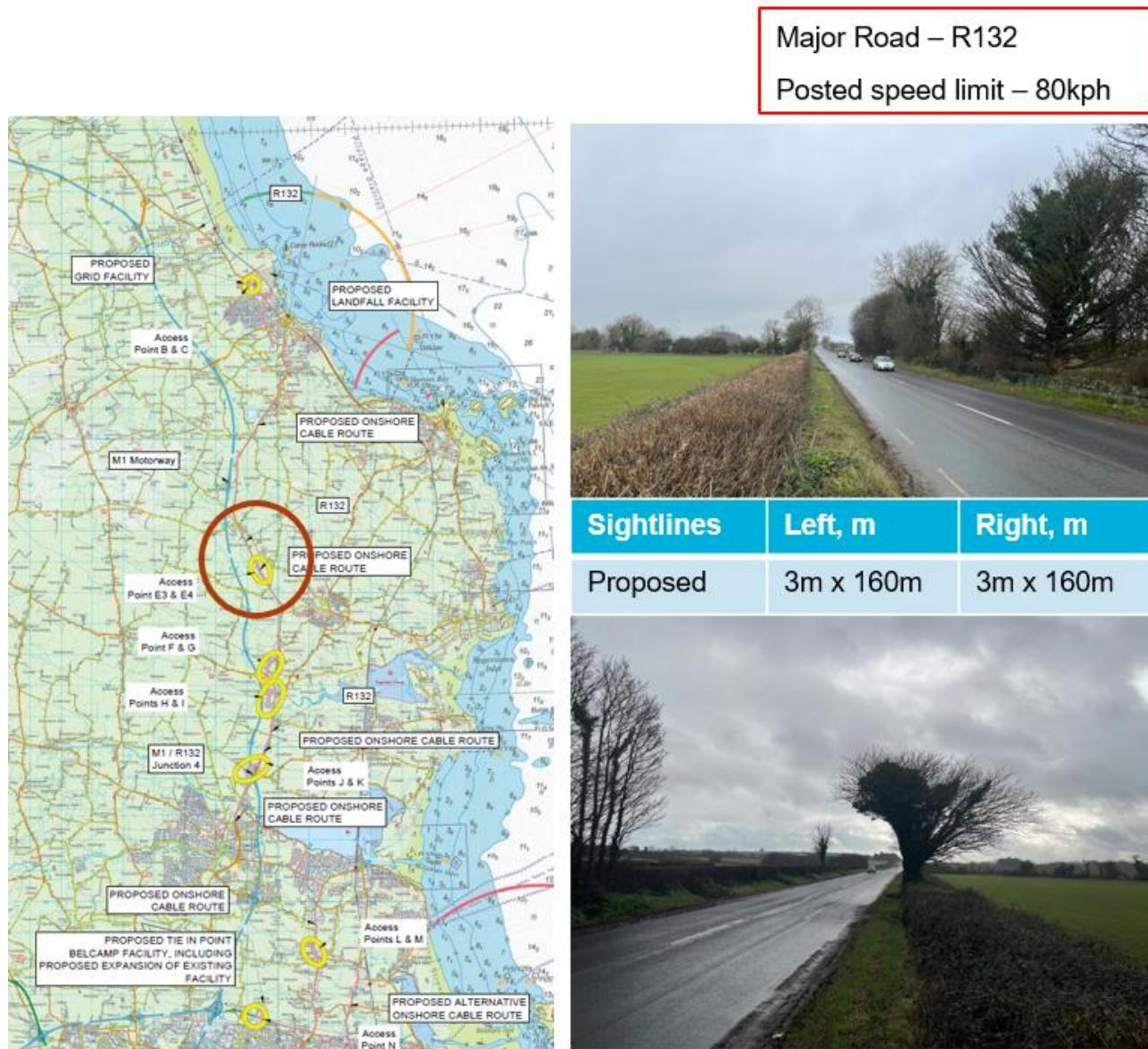
Figure 4.3 Location, photographs, applicable speed limits and sightlines for Access Point E3 to E4
