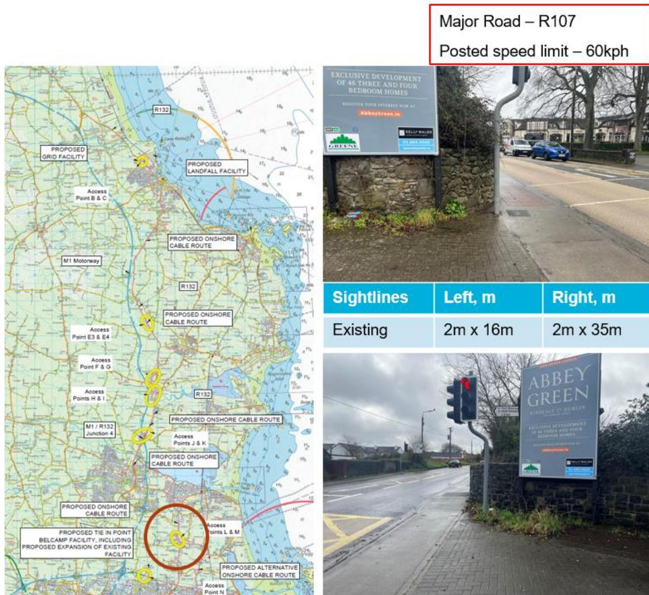
**Figure 4.11 Location, photographs, applicable speed limits and sightlines for Access Point M**
