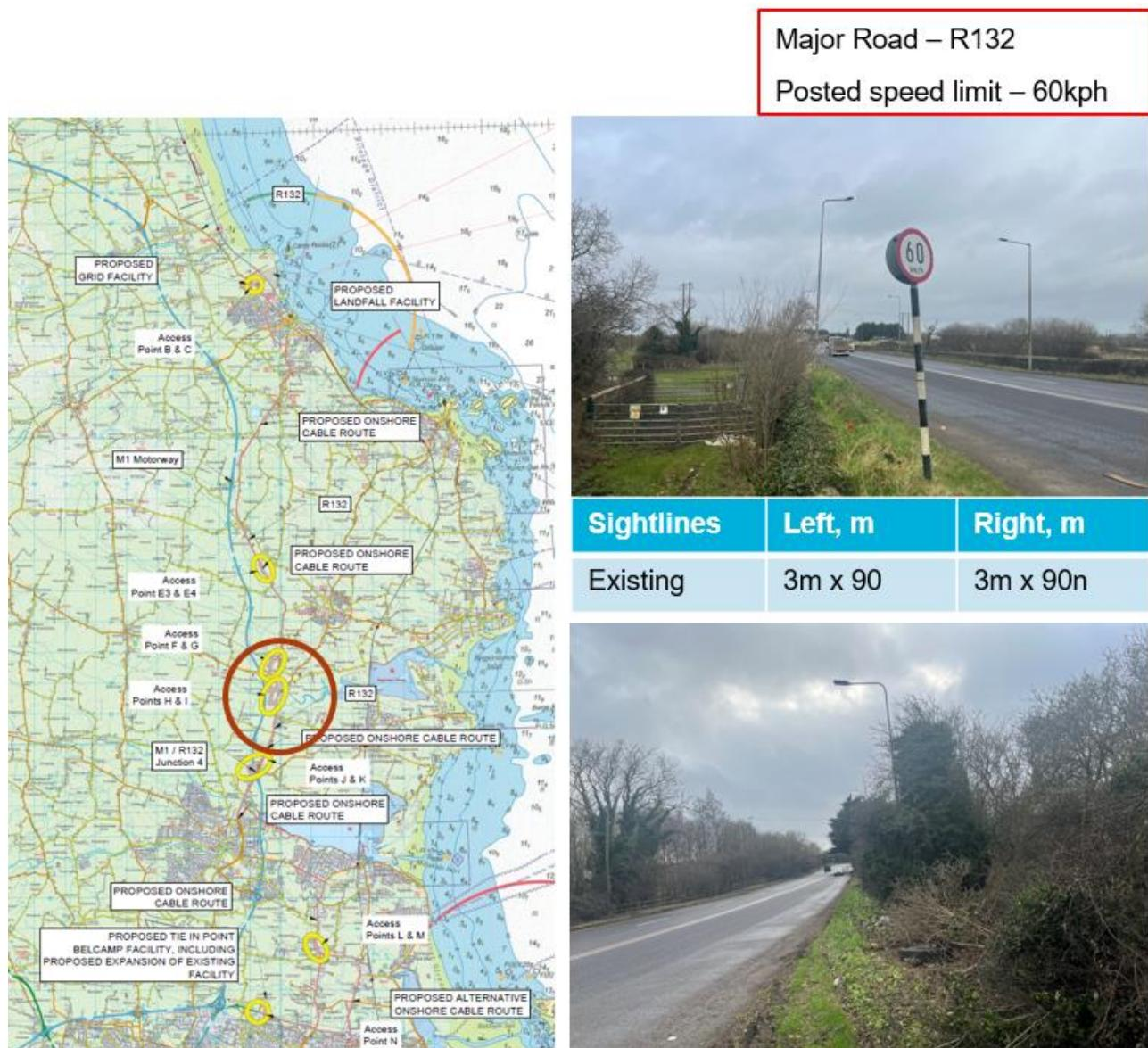
Figure 4.7 Location, photographs, applicable speed limits and sightlines for Access Point I
