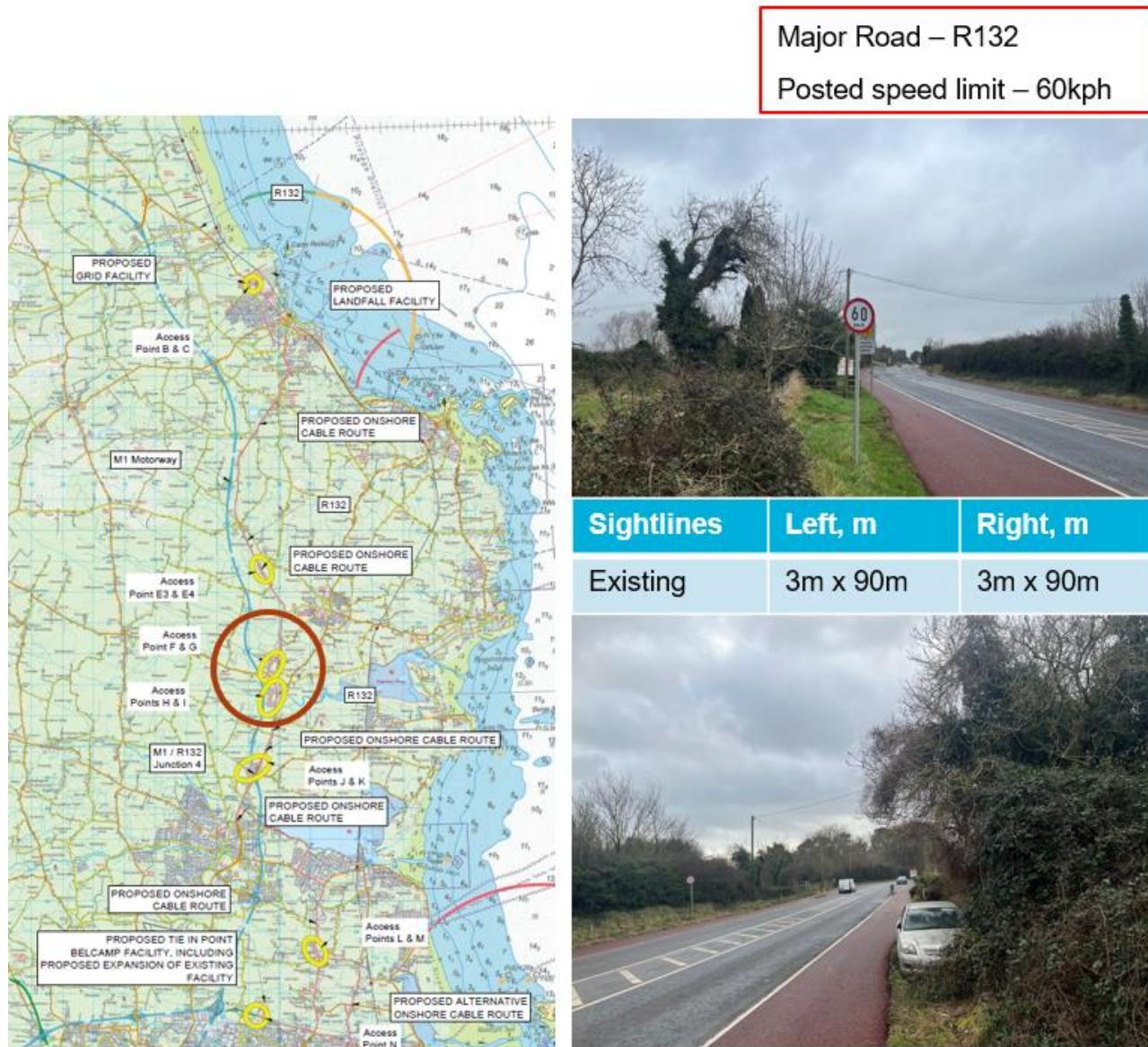
**Figure 4.4 Location, photographs, applicable speed limits and sightlines for Access Point F**
